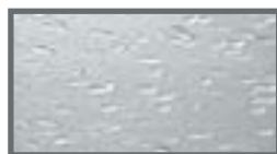
Hammered Etched Anodized Hammered Mill Finish (HEA)(HMF)
